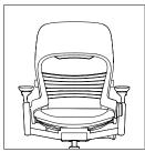
**Parallel slats** in the Live-Back shell provide extensive flexibility to allow back to conform to individual users.
