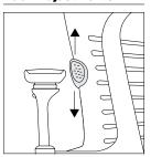
Lumbar height adjusts 5" (51/4" to 101/4" from seat. 61/2" to 111/2" on Plus chairs) by grabbing exposed tabs and sliding the lumbar support up or down. This feature is standard on work chairs and stools, but may be omitted.
